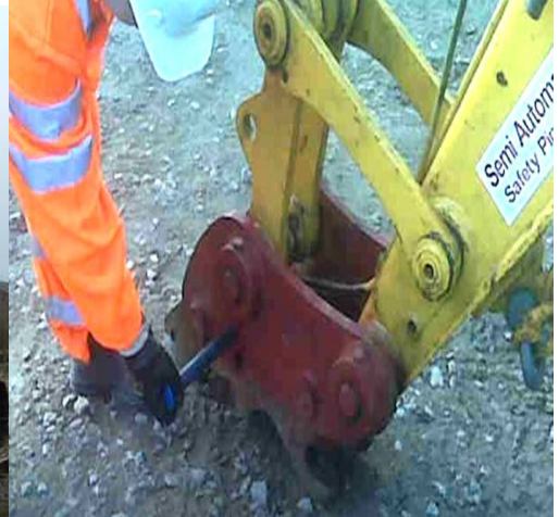
The RRV operator inserting the safety pin in a Semi automatic Quick Hitch
