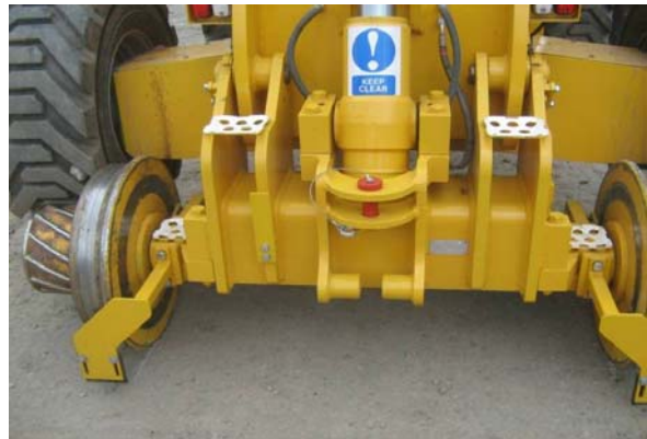
Braked axle, note inner face of rail wheel where the brake pad reacts.
